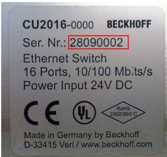
Fig. 3: CU2016 switch with serial/ batch number
