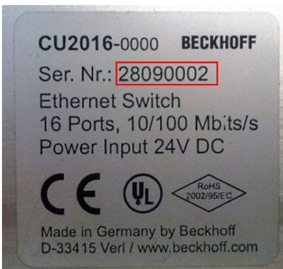
Fig. 3: CU2016 switch with serial/ batch number
