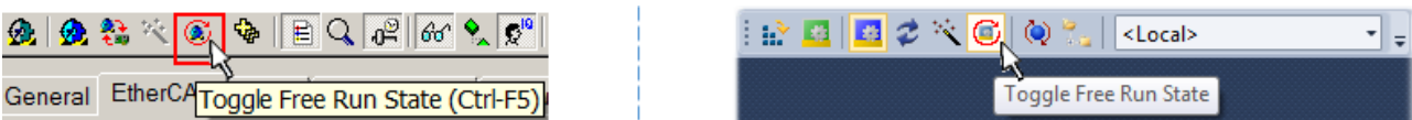
Fig. 118: TwinCAT can also be switched to this state by using a button (left: TwinCAT 2; right: TwinCAT 3)
