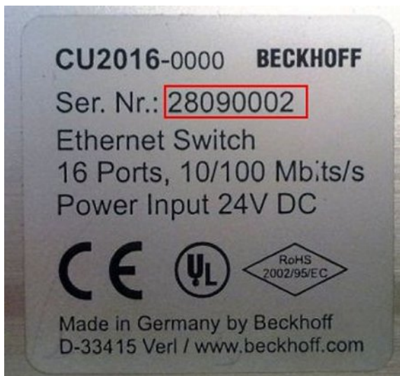
Fig. 3: CU2016 switch with serial/ batch number
