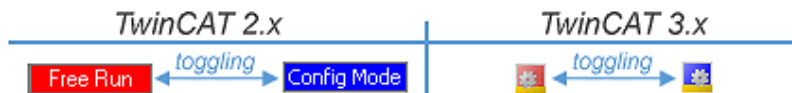
Fig. 125: Displaying of “Free Run” and “Config Mode” toggling right below in the status bar
