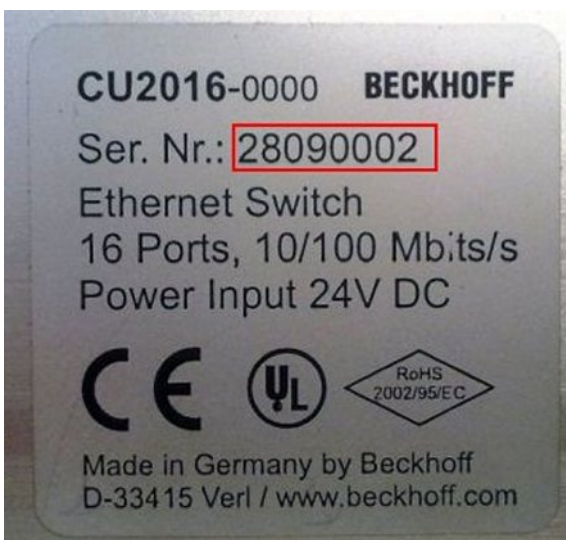
Fig. 3: CU2016 switch with serial/ batch number
