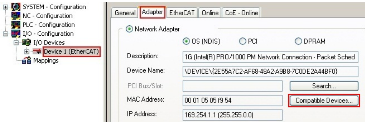
Fig. 63: EtherCAT device properties(TwinCAT 2): click on „Compatible Devices...“ of tab “Adapter”
