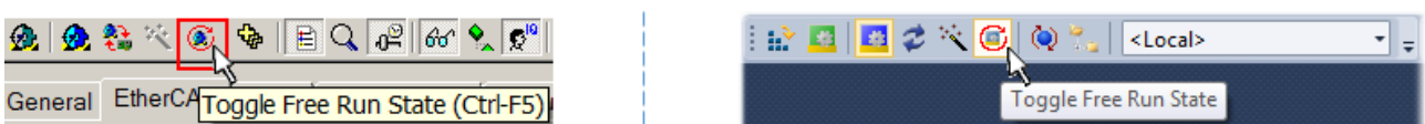
Fig. 96: TwinCAT can also be switched to this state by using a button (left: TwinCAT 2; right: TwinCAT 3)
