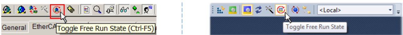
Fig. 117: TwinCAT can also be switched to this state by using a button (left: TwinCAT 2; right: TwinCAT 3)
