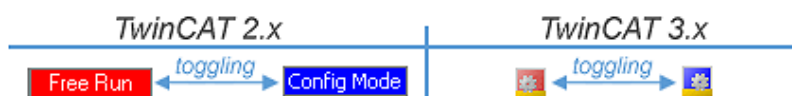
Fig. 98: Displaying of “Free Run” and “Config Mode” toggling right below in the status bar
