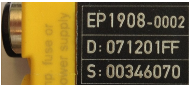
Fig. 6: EP1908-0002 IP67 EtherCAT Safety Box with batch number 071201FF and unique serial number 00346070
