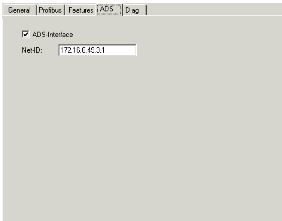
Fig. 126: DP master, ADS tab: Activating the ADS interface and entering the Net ID
