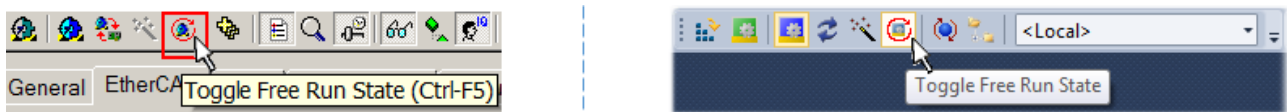
Fig. 67: TwinCAT can also be switched to this state by using a button (left: TwinCAT 2; right: TwinCAT 3)
