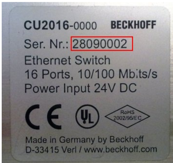
Fig. 3: CU2016 switch with batch number
