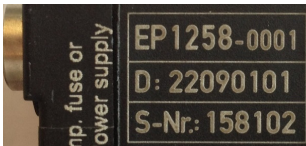
Fig. 5: EP1258-00001 IP67 EtherCAT Box with batch number 22090101 and unique serial number 158102
