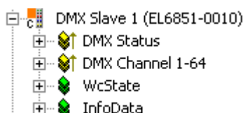
Fig. 130: TwinCAT tree DMX slave, process image up to 64 bytes of user data
