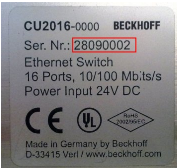
Fig. 3: CU2016 switch with batch number
