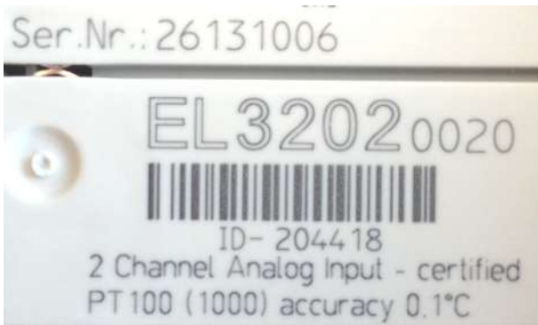
Fig. 4: EL3202-0020 with batch numbers 26131006 and unique ID-number 204418
