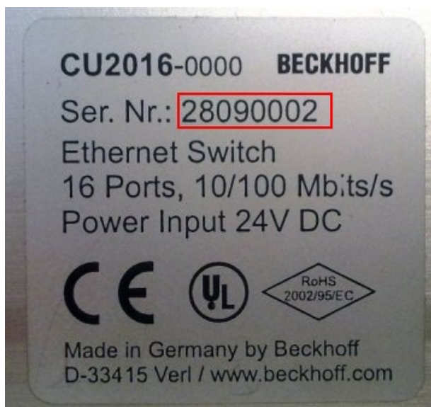
Fig. 3: CU2016 switch with batch number
