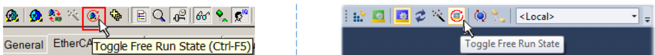
Fig. 119: TwinCAT can also be switched to this state by using a button (left: TwinCAT 2; right: TwinCAT 3)
