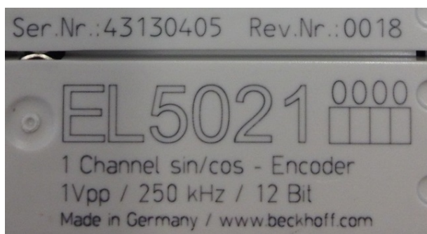
Fig. 1: EL5021 EL terminal, standard IP20 IO device with batch number and revision ID (since 2014/01)
