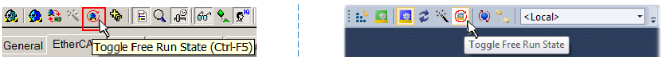
Fig. 110: TwinCAT can also be switched to this state by using a button (left: TwinCAT 2; right: TwinCAT 3)
