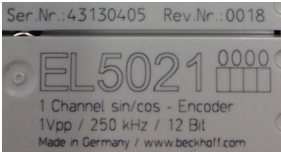
Fig. 2: EL5021 EL terminal, standard IP20 IO device with serial/ batch number and revision ID (since 2014/01)
