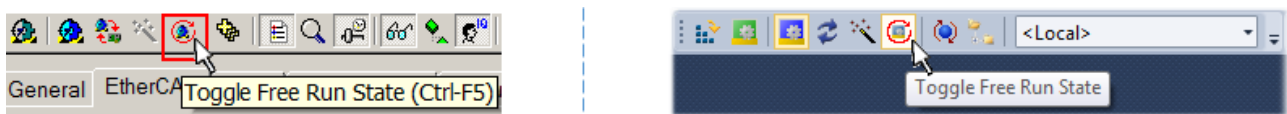
Fig. 68: TwinCAT can also be switched to this state by using a button (left: TwinCAT 2; right: TwinCAT 3)
