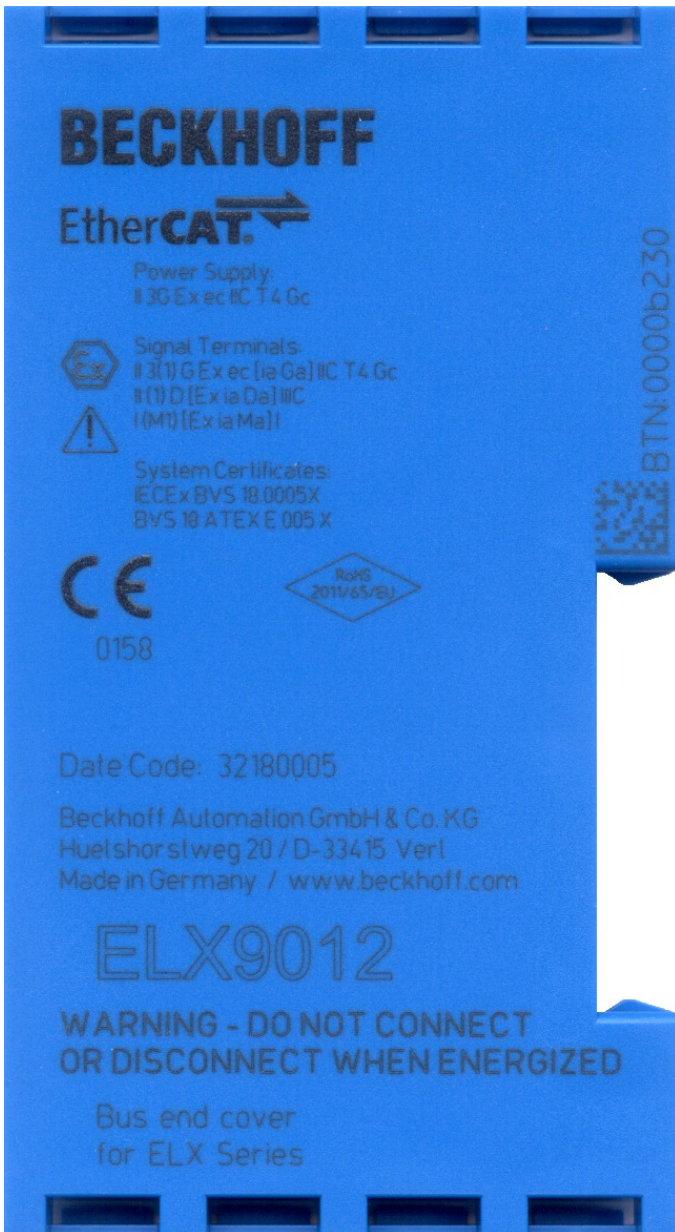
Fig. 2: ELX9012 with date code 32180005 and Ex marking
