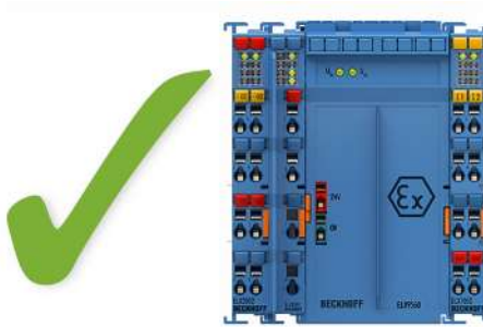
Fig. 9: Valid arrangement - ELX9410 in front of an ELX9560 power supply terminal.
