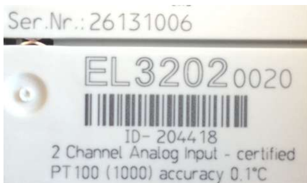
Fig. 4: EL3202-0020 with batch numbers 26131006 and unique ID-number 204418
