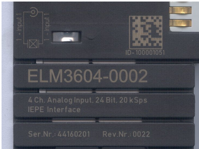
Fig. 8: ELM3604-0002 terminal with ID number (QR code) 100001051 and unique serial number 44160201
