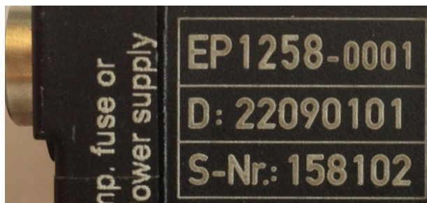
Fig. 5: EP1258-0001 IP67 EtherCAT Box with batch number 22090101 and unique serial number 158102
