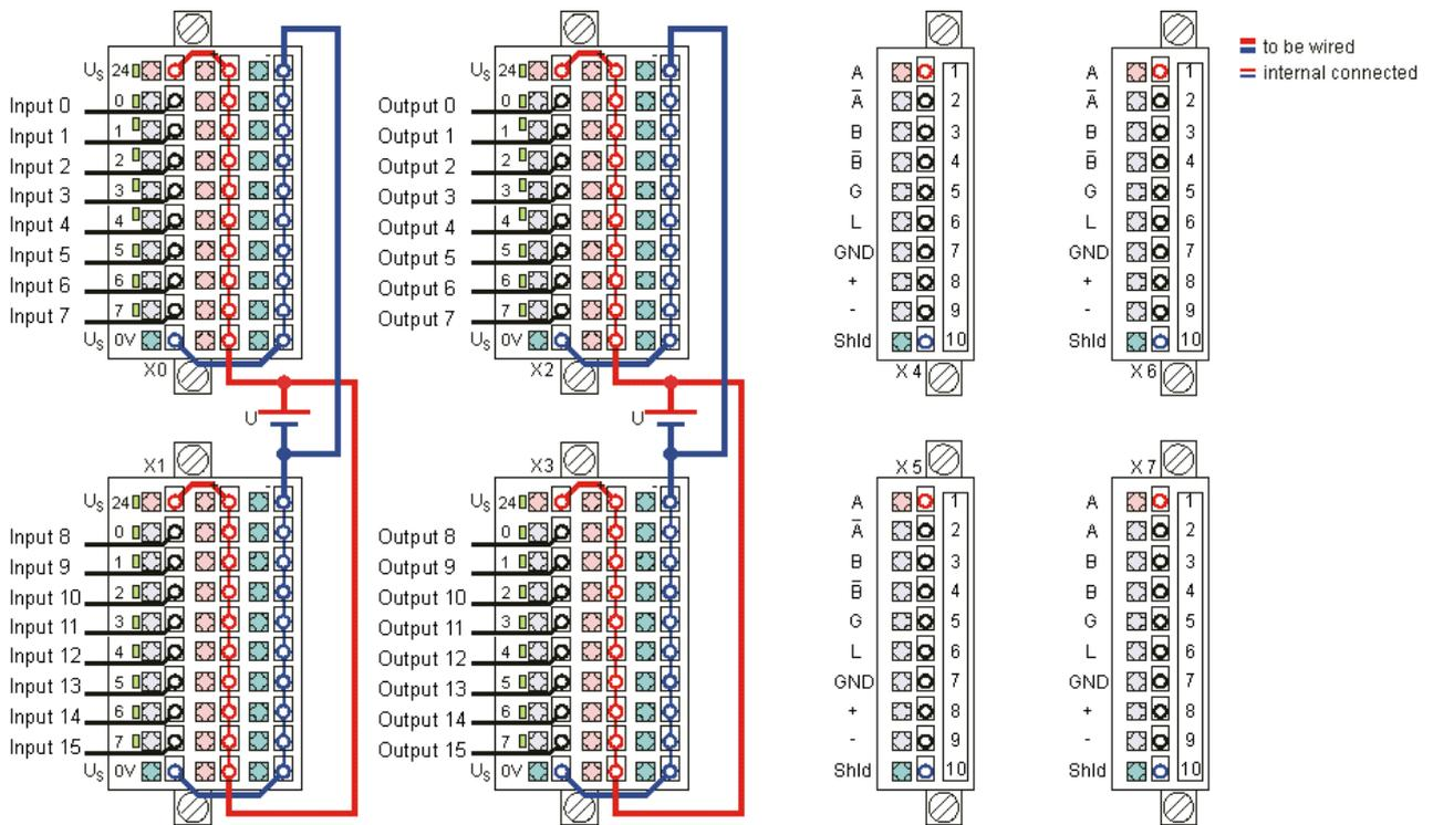
Fig. 20: Connection of the module with alternative power supply
