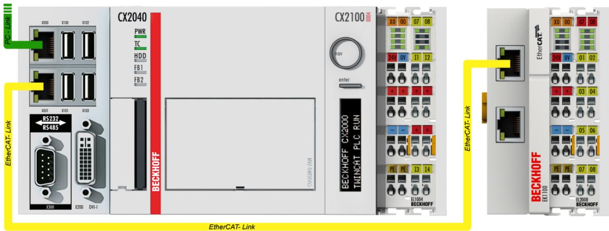
Fig. 24: Control configuration with an Embedded PC and input (EL1004) and output (EL2008)
