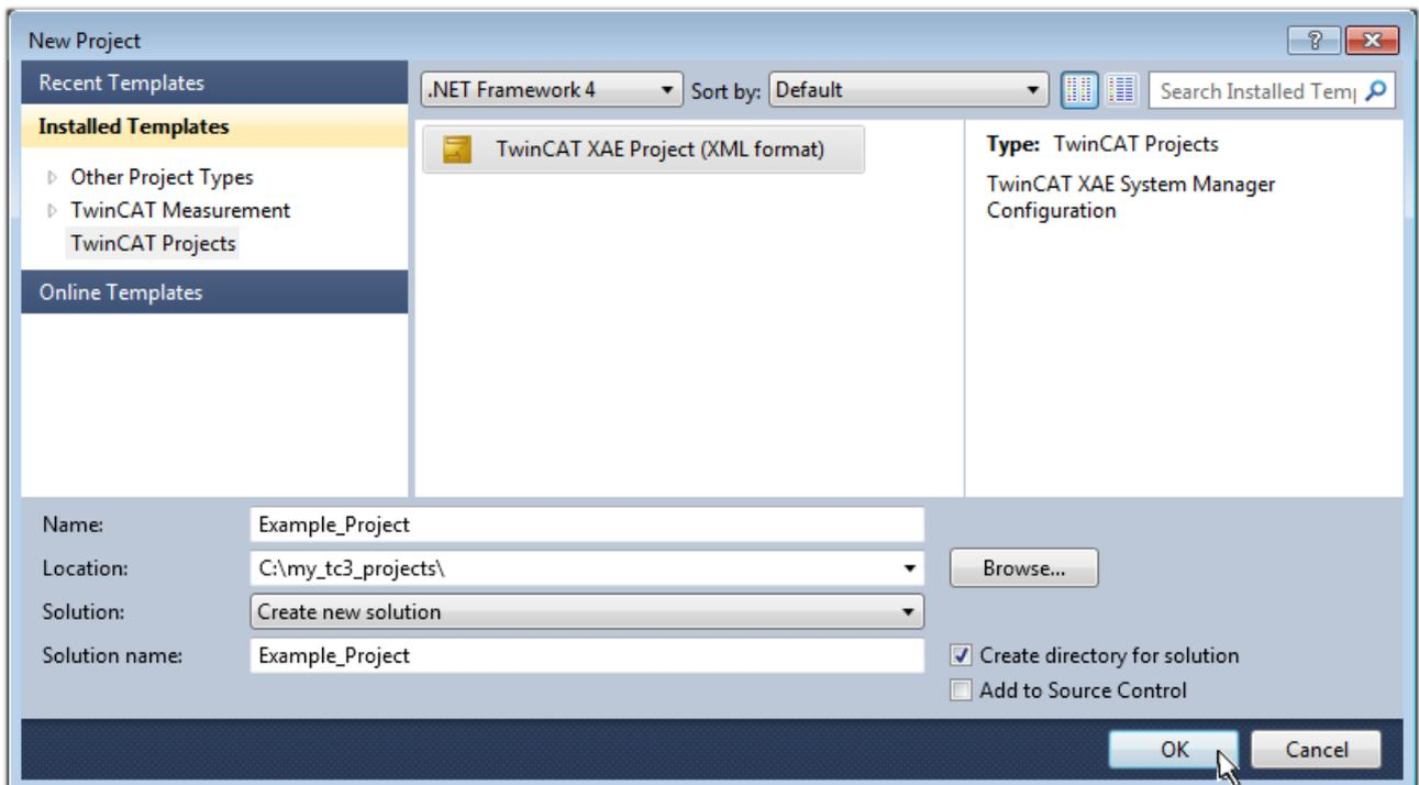
Fig. 43: Create new TwinCAT project
