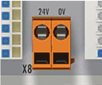
Fig. 19: Clamped joint for power supply
