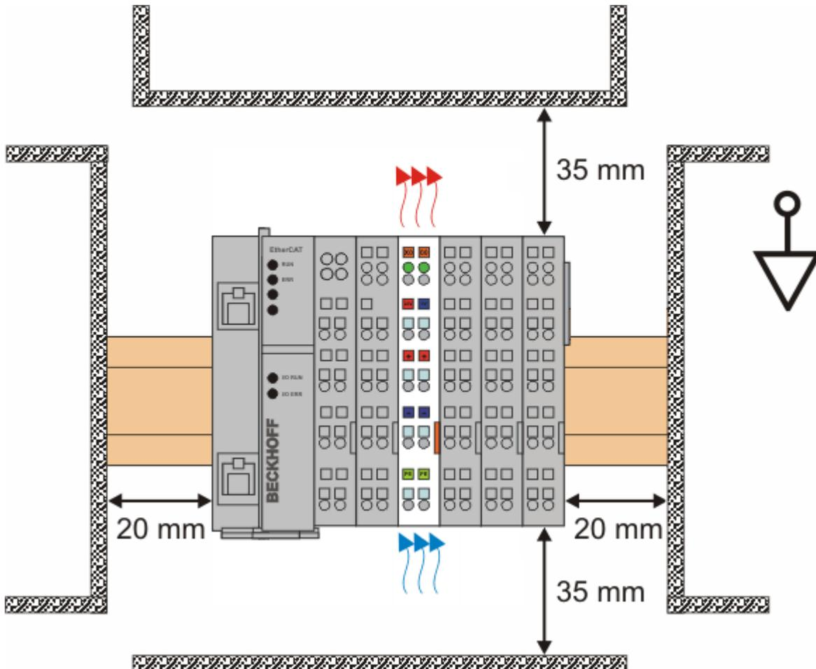
Fig. 17: Recommended distances for standard installation position
