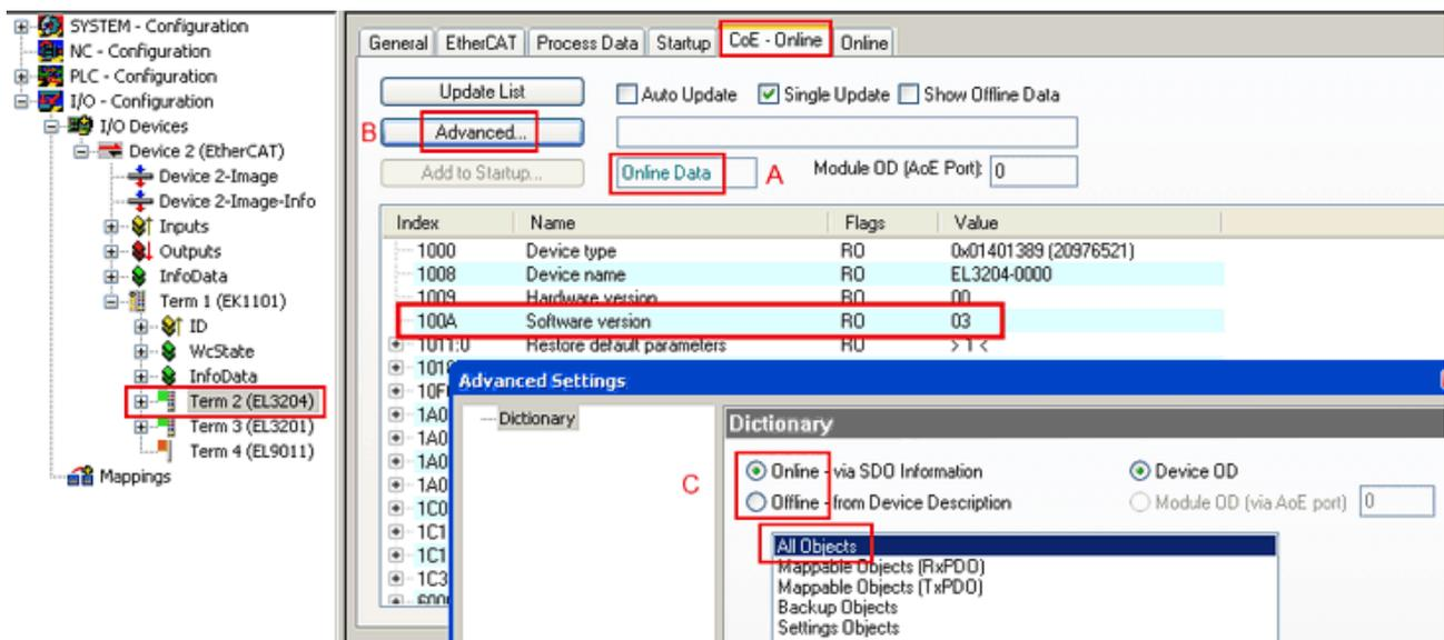
Fig. 136: Display of EL3204 firmware version
