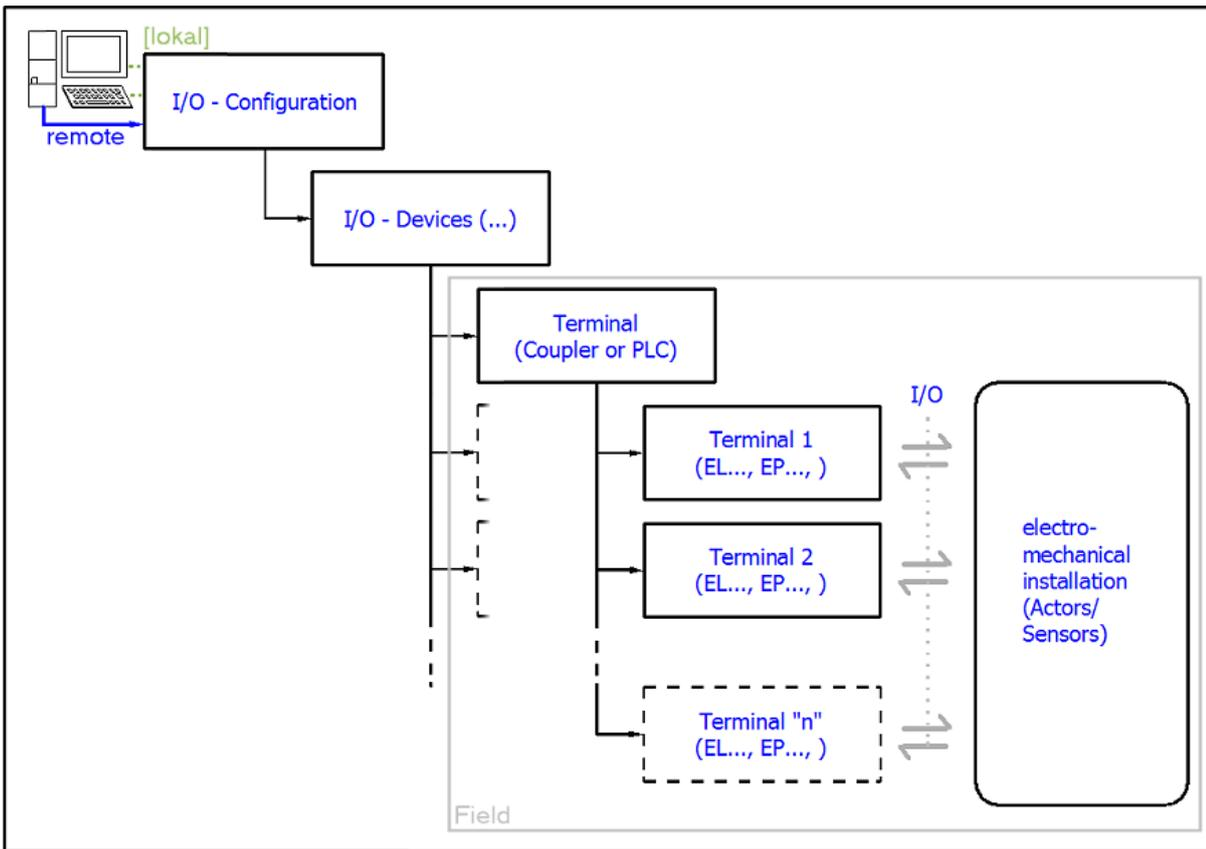
Fig. 23: Relationship between user side (commissioning) and installation
