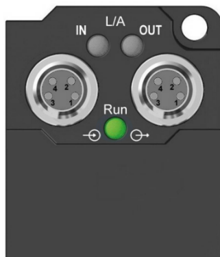
Fig. 21: Run LED diagnostics
