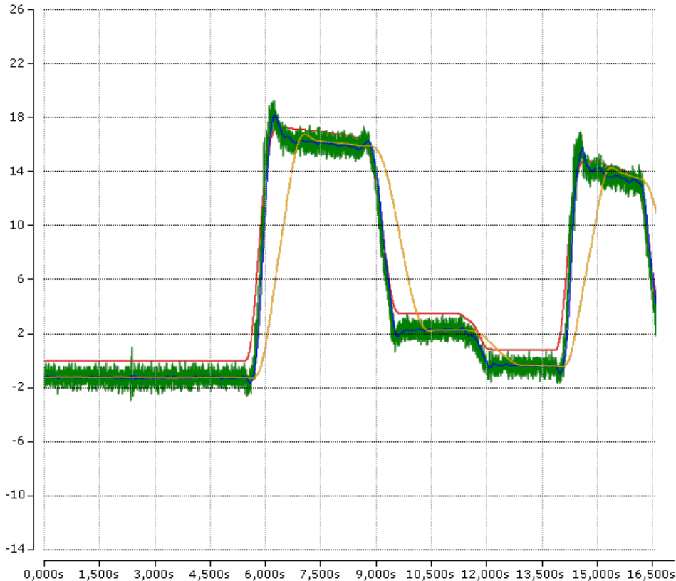
Fig. 30: Angle measurement, process data as acceleration values, calculation on a PC
