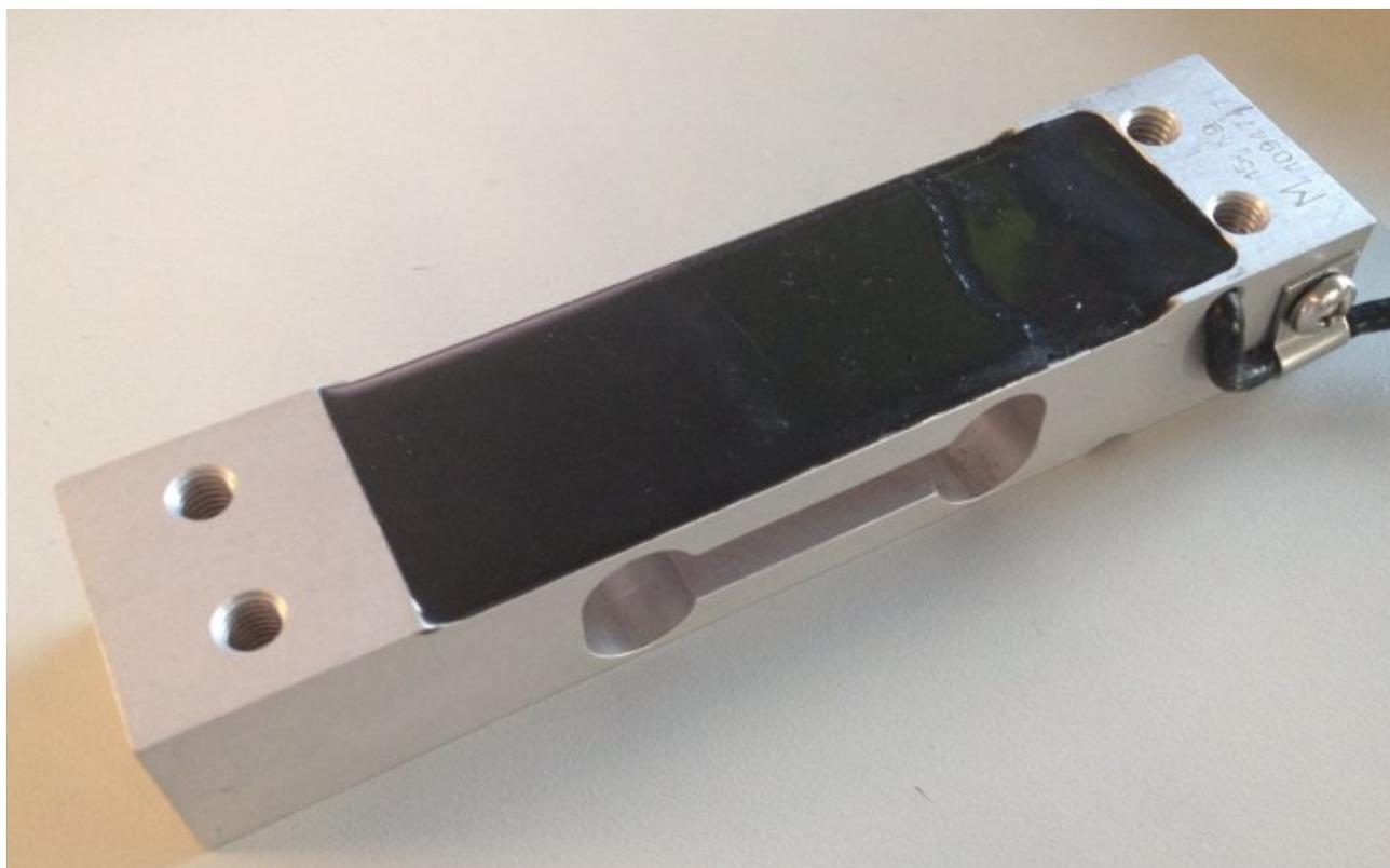
Fig. 6: Example of a load cell
