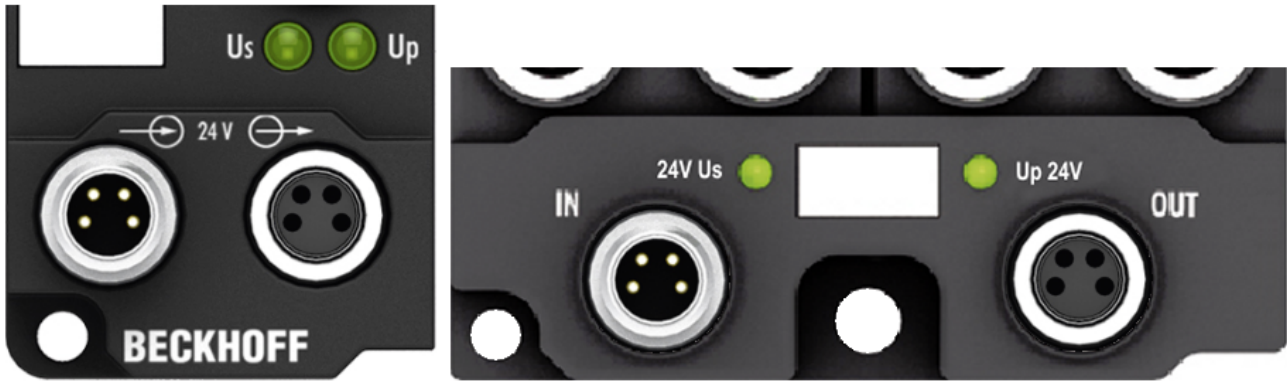
Fig. 18: EtherCAT Box, Connectors for power supply
