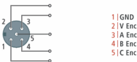
Fig. 29: Encoder connection
