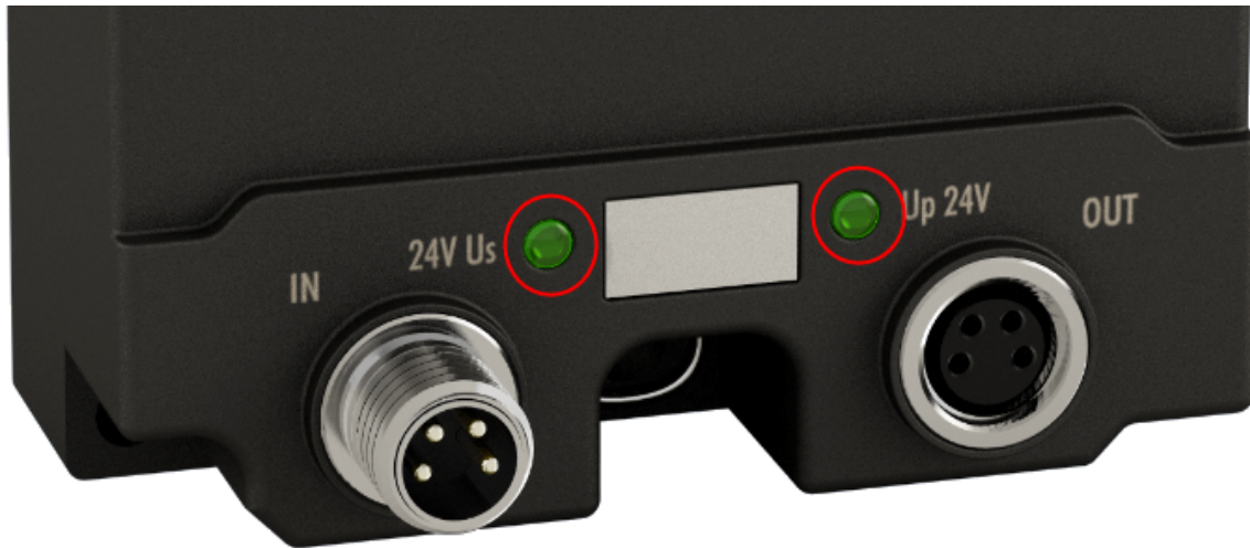
Fig. 19: LED display for the supply voltages
