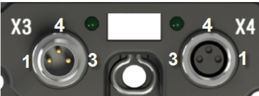
Fig. 28: EP9214 - Monitoring and reset contacts
