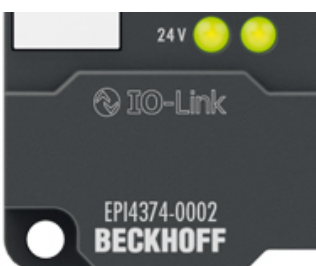
Fig. 15: Status LEDs for power supply
