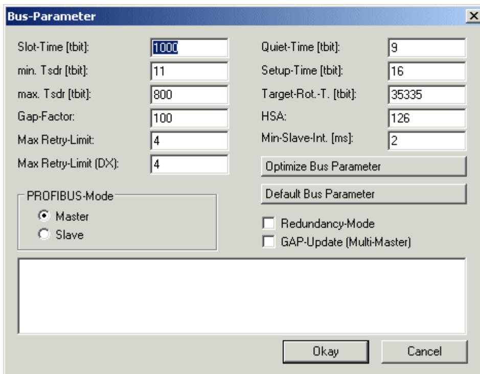
Fig. 27: TwinCAT 2.9 - Bus Parameters dialog
