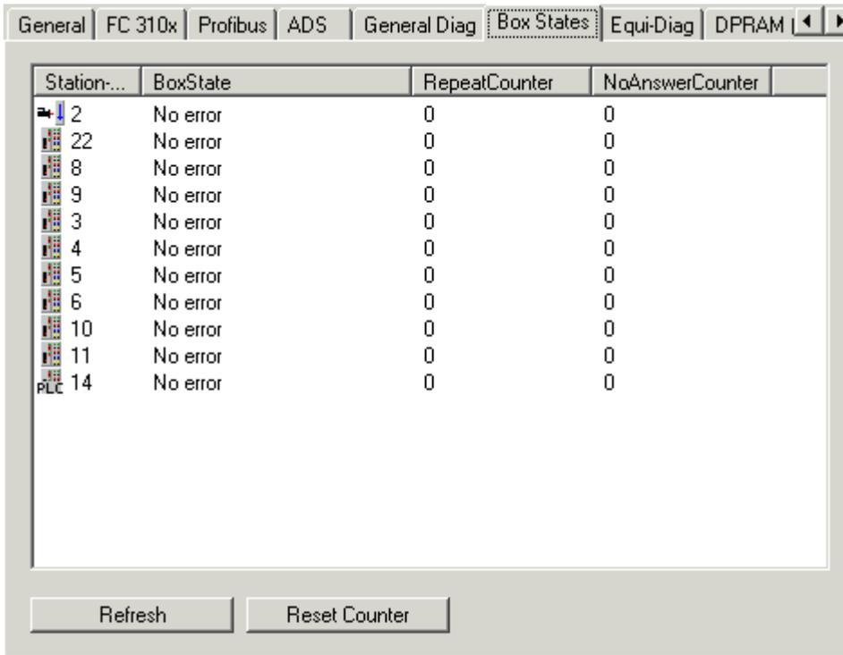
Fig. 32: TwinCAT 2.9 - Box States tab
