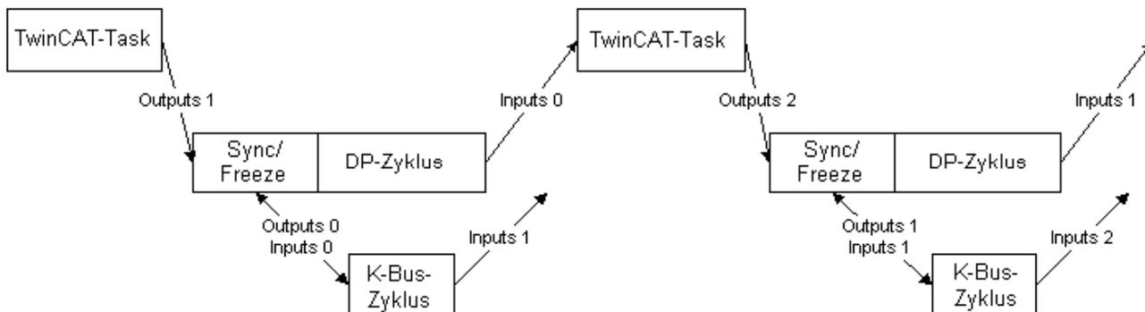
Fig. 9: Sync/Freeze functionality
