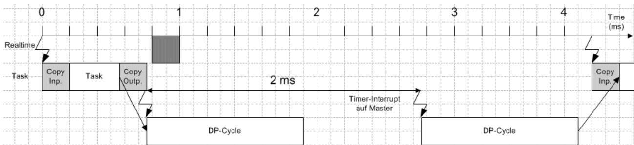
Fig. 7: Multiple DP Cycles in one Task Cycle
