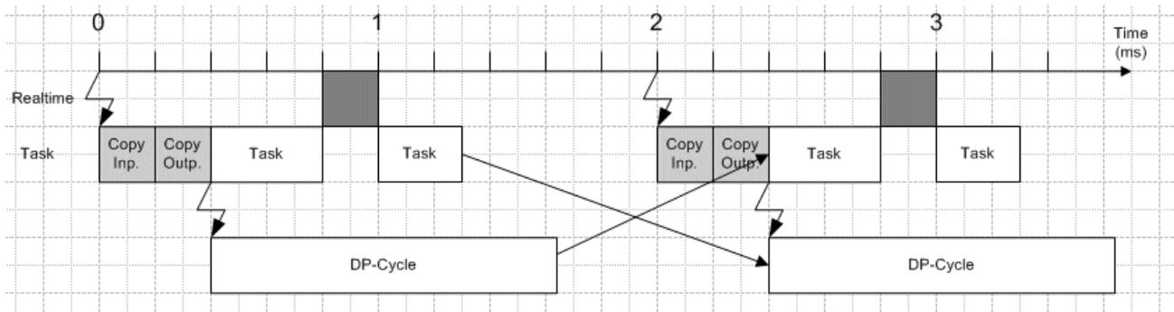
Fig. 3: I/O at task start and real-time resources exceeded
