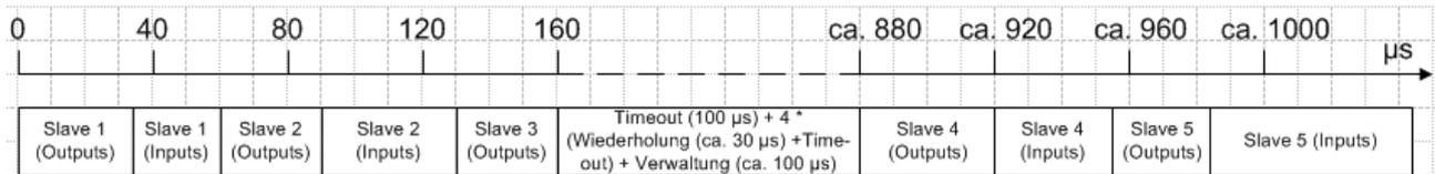
Fig. 11: First occurrence of a faulty DP cycle
