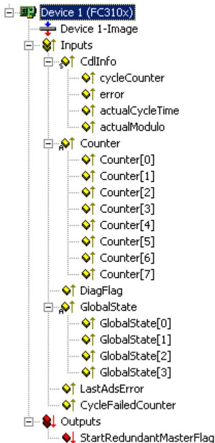
Fig. 15: Diagnostic variables of the PROFIBUS master
