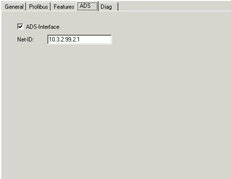
Fig. 43: Enabling the ADS interface on the DP master
