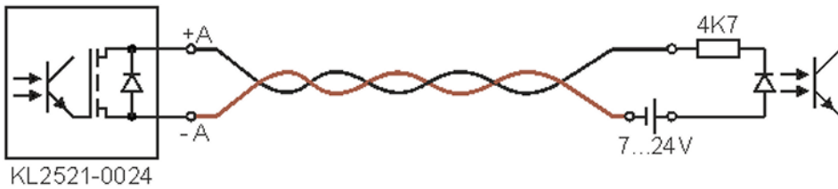
Fig. 16: KL2521-0024 - wiring with external power source
