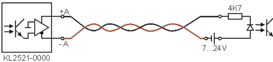
Fig. 15: KL2521-0000 up to hardware version 03 - wiring with external power source
