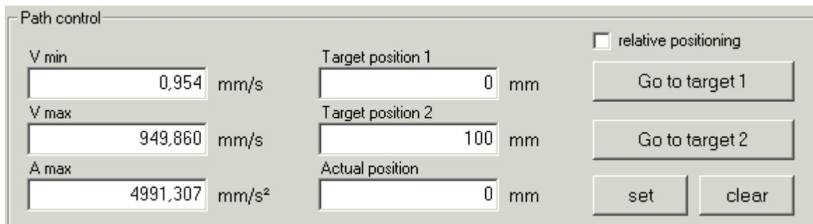
Fig. 42: Setting the path control in the *Commissioning* tab
