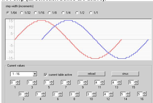
Fig. 34: KL2541 - Examples for current table settings with KS2000
