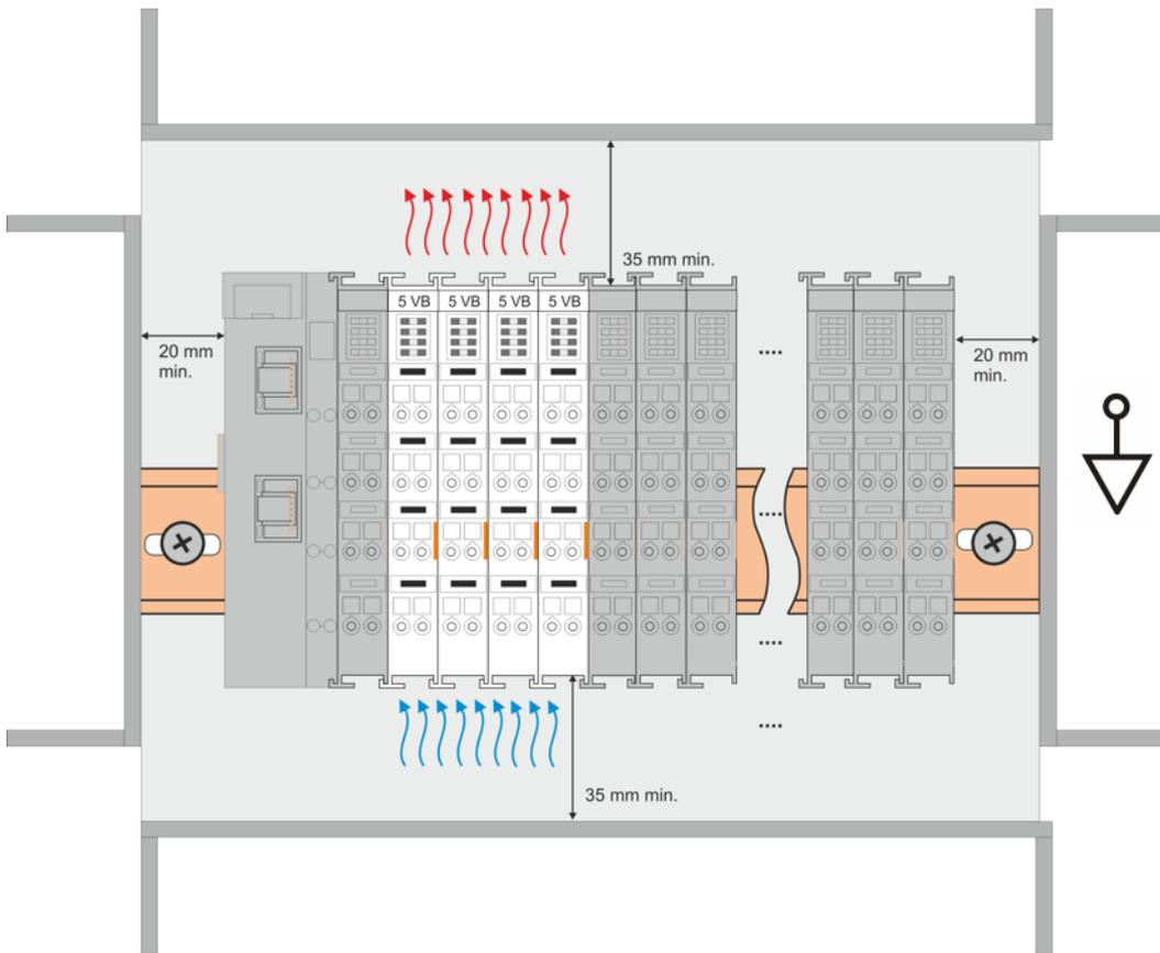
Fig. 12: Recommended distances of installation position for operating without fan
