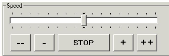
Fig. 41: Setting the velocity in the *Commissioning* tab
