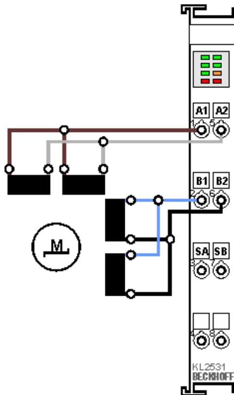
Fig. 21: KL2531 - Bipolar serial (left) and parallel (right) control of a bipolar motor
