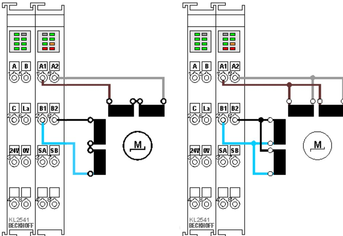
Fig. 24: KL2541 - Bipolar serial (left) and parallel (right) control of a bipolar motor
