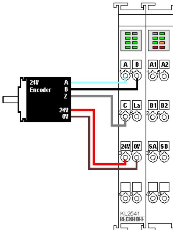
Fig. 26: KL2541 - Connecting an encoder
