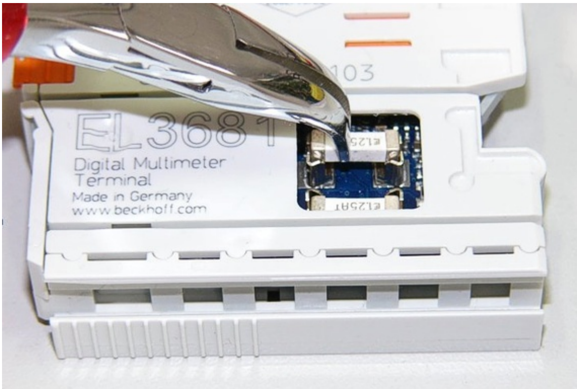
Fig. 20: Replacing the fuse
