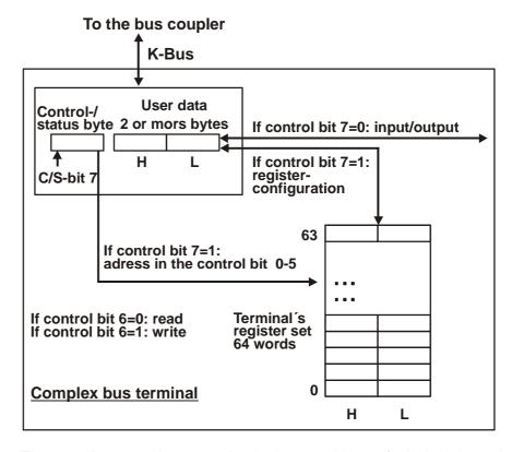
The control or status byte occupies the lowest address of a logical channel. The corresponding register values are located in the following 2 data bytes (the BK2000 is an exception to the rule: here, an unused data byte is inserted after the control or status byte, thus setting the register value to a word limit).
