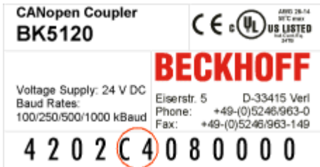
Fig. 30: Specification of the firmware version on a Bus Coupler
