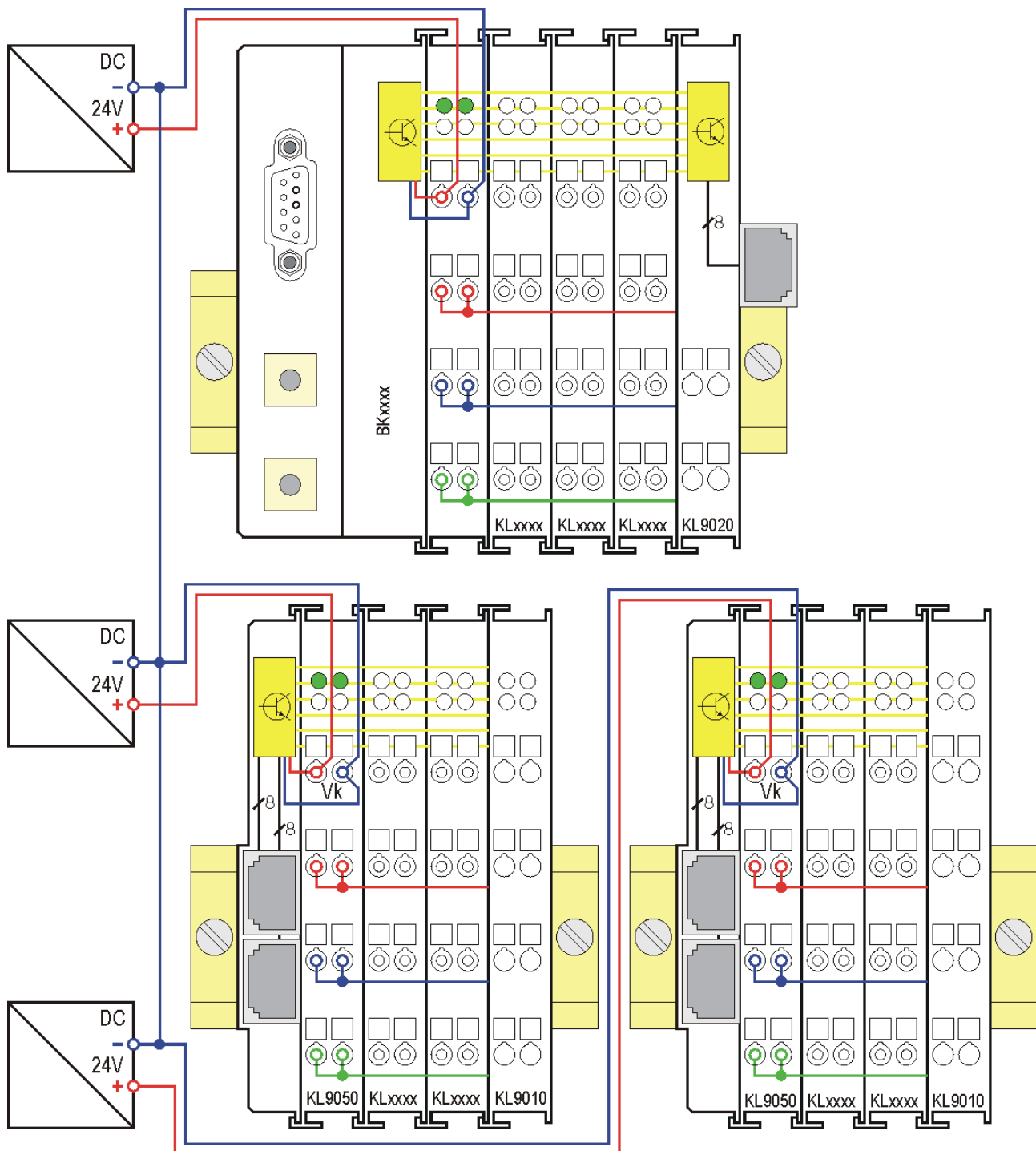
Fig. 14: KL9020, KL9050 – Connection of the power supply
