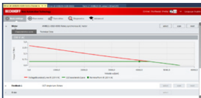
Detailed visualisation of the motor characteristic according to the electronic identification plate
