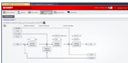
Direct fine-tuning of the drive during commissioning
