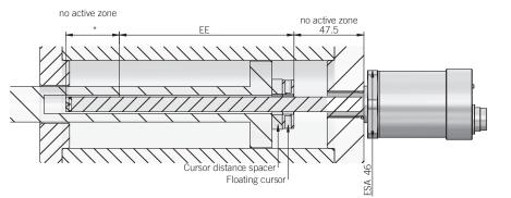
\* = 55 mm up to stroke 1000 mm, from 1250 mm consider 60 mm due to M4 threaded hole
