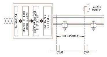
SSI output goes to 0 if the echo is absent (magnet out of measurement range or internal device error)
