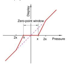
It makes sense to set the *Offset* (zero-point displacement) if, without pressure (remove measuring line), the display shows a value that is not zero. Be-
