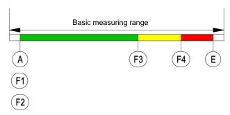
The parameter *Hysteresis* can be used to prevent fast and unwanted colour changes. The hysteresis is set in the range 0.1... 10%.
