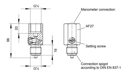
Fig. 8: Damping reactor MZ410#
