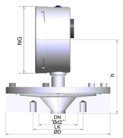
Fig. 15: Connection flange
