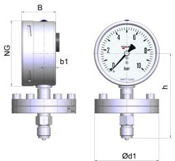
Fig. 12: Dimension drawing MA15F without contacts
