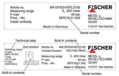
Fig. 3: Type plates with and without contacts
