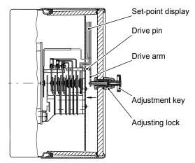
Fig. 11: Contact element
