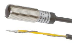
its status. 3. With the diffuse reflection sensor, the transmitter and receiver are in one device. The emitted light beam is reflected by the object that is to be detected. As soon as the receiver detects the reflected light, the switching output integrated in the device changes its status.
