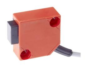
its status. 3. With the diffuse reflection sensor, the transmitter and receiver are in one device. The emitted light beam is reflected by the object that is to be detected. As soon as the receiver detects the reflected light, the switching output integrated in the device changes its status.
