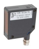
its status. 3. With the diffuse reflection sensor, the transmitter and receiver are in one device. The emitted light beam is reflected by the object that is to be detected. As soon as the receiver detects the reflected light, the switching output integrated in the device changes its status.
