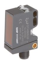
its status. 3. With the diffuse reflection sensor, the transmitter and receiver are in one device. The emitted light beam is reflected by the object that is to be detected. As soon as the receiver detects the reflected light, the switching output integrated in the device changes its status.
