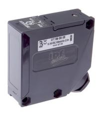
its status. 3. With the diffuse reflection sensor, the transmitter and receiver are in one device. The emitted light beam is reflected by the object that is to be detected. As soon as the receiver detects the reflected light, the switching output integrated in the device changes its status.
