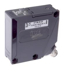
its status. 3. With the diffuse reflection sensor, the transmitter and receiver are in one device. The emitted light beam is reflected by the object that is to be detected. As soon as the receiver detects the reflected light, the switching output integrated in the device changes its status.
