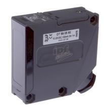
its status. 3. With the diffuse reflection sensor, the transmitter and receiver are in one device. The emitted light beam is reflected by the object that is to be detected. As soon as the receiver detects the reflected light, the switching output integrated in the device changes its status.
