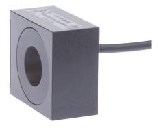
its status. 3. With the diffuse reflection sensor, the transmitter and receiver are in one device. The emitted light beam is reflected by the object that is to be detected. As soon as the receiver detects the reflected light, the switching output integrated in the device changes its status.
