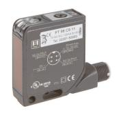
its status. 3. With the diffuse reflection sensor, the transmitter and receiver are in one device. The emitted light beam is reflected by the object that is to be detected. As soon as the receiver detects the reflected light, the switching output integrated in the device changes its status.
