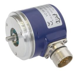
encoder shaft can be equipped with measuring wheels or pinions in various designs and sizes. Typical applications include the angle measurement on bending machines, length measuring of belt systems or speed measurement on winding systems.
