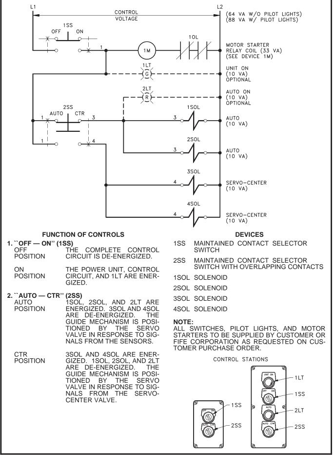
AUTO-CENTER CONTROL SYSTEM FOR FIXED SENSOR CENTERGUIDE WITH MODEL SM-1760 SENSORS
