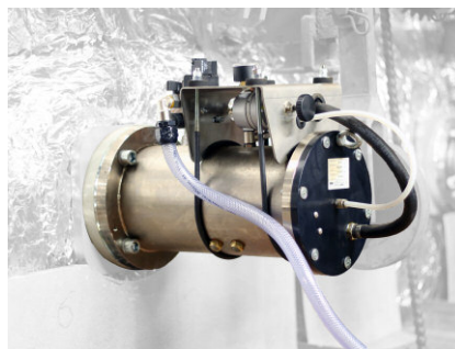
NHK for cleaning the harp of a heat exchanger
